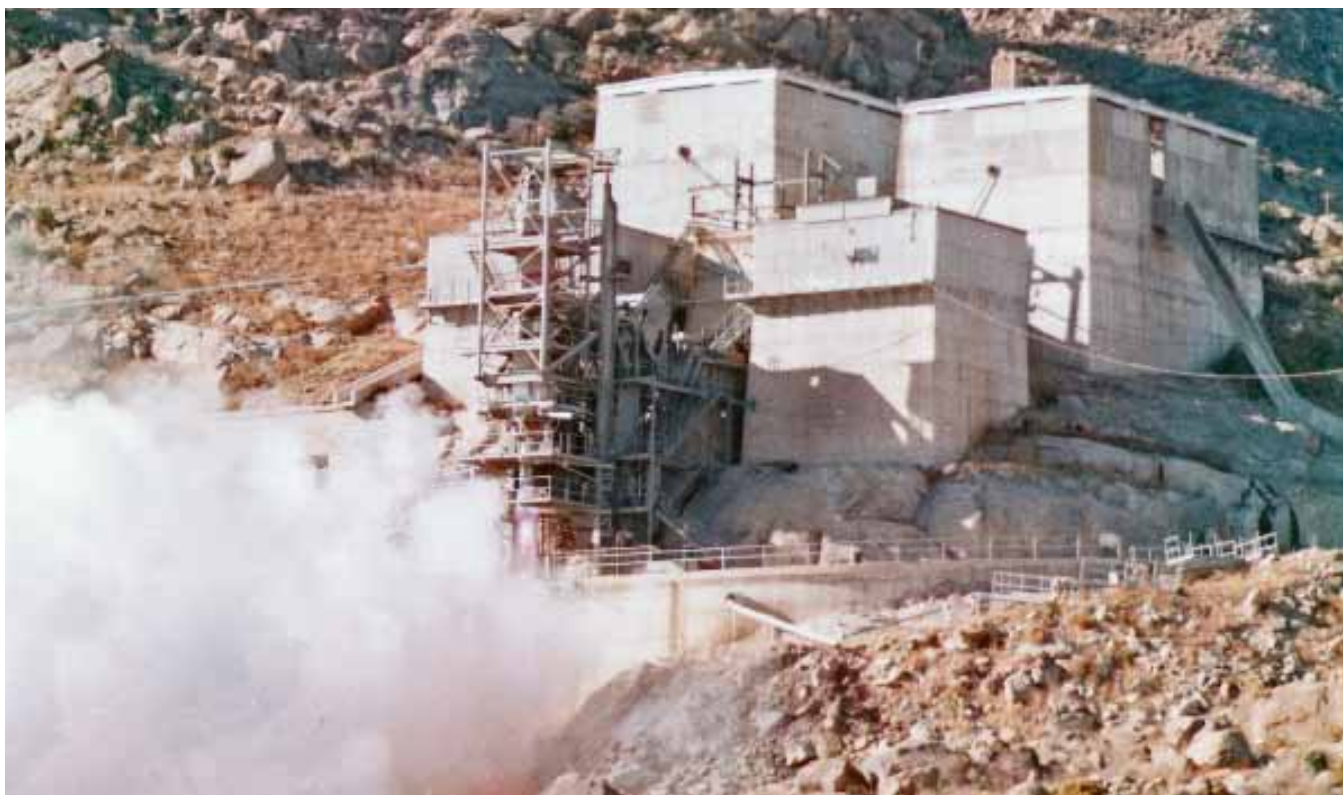
A Redstone motor under test at the 500K Static Test Stand. As you drive along War Road and look at 500K, it appears there is a tunnel below the stand. That is an area that has been hollowed out by the super hot exhaust gases from the tests hitting the granite and then the spray of water from above to cool everything. Yards of rock have spalled off the face over the years creating an alcove under the facility. Courtesy photo
